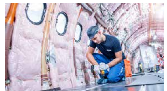
Installation of a replacement floor panel
