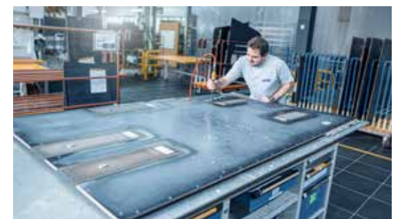
Precision work during assembly of VAP beams into floor panels
