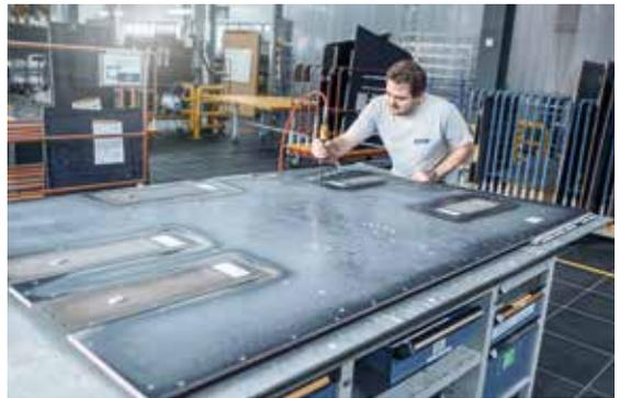
Precision work during assembly of VAP beams into floor panels
