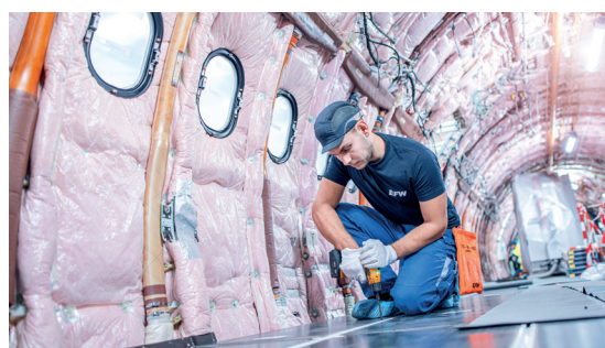
Installation of a replacement floor panel
