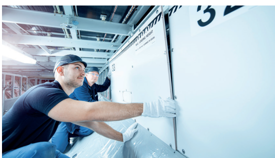
Installation of a replacement lining panel
