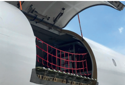
MAIN DECK CARGO DOOR 142" width and 85" height clearance, hydraulically actuated and electrically locked
