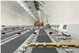
MANUAL CARGO LOADING SYSTEM Full support of industry standard narrowbody ULDs
